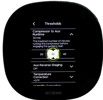
Compressor to Aux Runtime - 30 min
